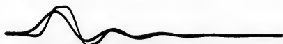
Fig. 14. Normal and crispened \frac{1}{8} -msec pulse waveforms for a system of 2-mc bandwidth to the 3-db point.
